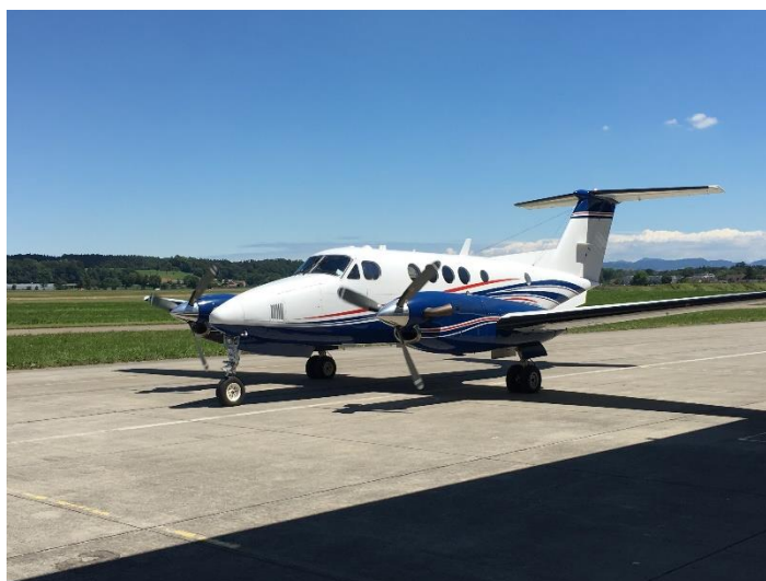
Figure 1 A King Air B200 is used as airborne platform for AVIRIS-NG.
